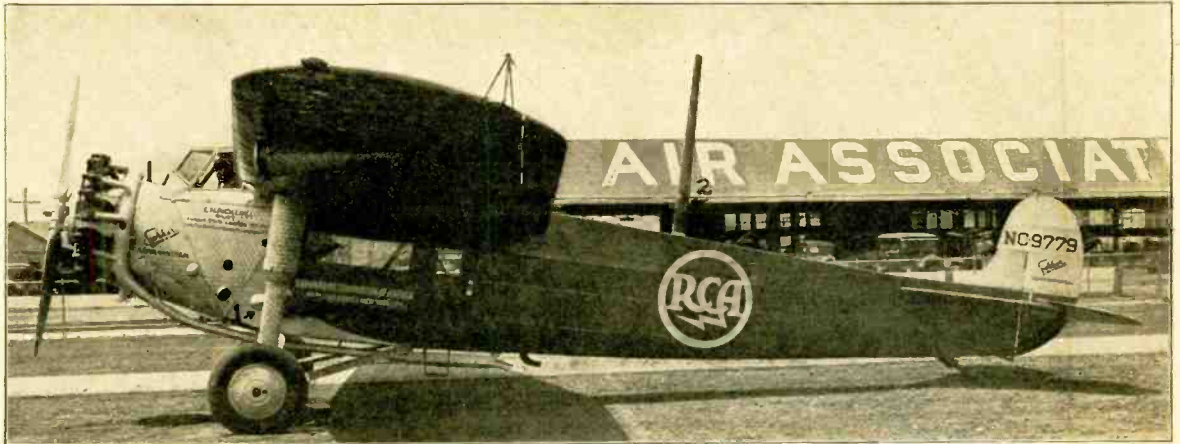
The experimental flying radio laboratory of the Radiomarine Corp., of America, is shown above. The black arrow shown near one of the landing struts indicates the wind-driven dynamo, which supplies the current for the radio transmitter.
