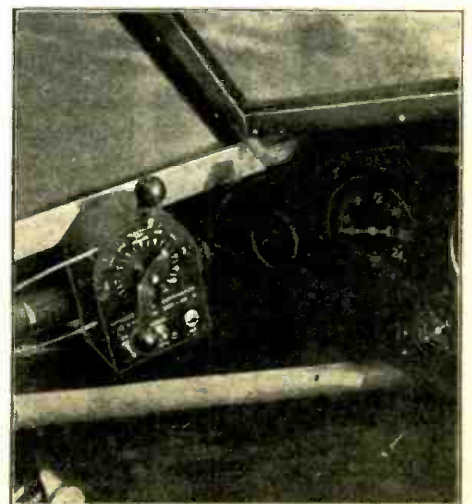
Close-up of the remote volume and tuning controls for use with Stromberg-Carlson aircraft radio receiver.
